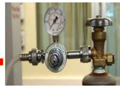
Connect the Heliox regulator to the tank.
