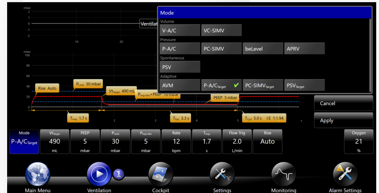
TargetVent modes available and the new ventilation mode table for better visibility in 6.1
